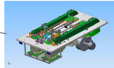
All tooling is mounted to a substantial aluminium base plate, this provides an excellent stable platform for the high speed operation.
