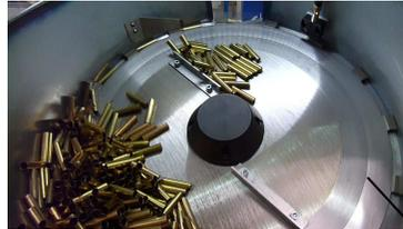
The machine can easily handle multi calibre and ball and blank rounds with simple tooling change.
