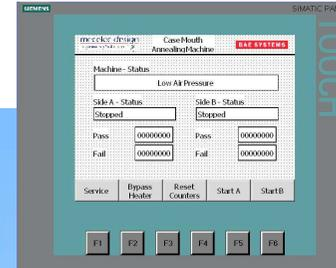
The test rig is controlled by a Siemens S7-300 PLC with a 8" touchscreen HMI.
